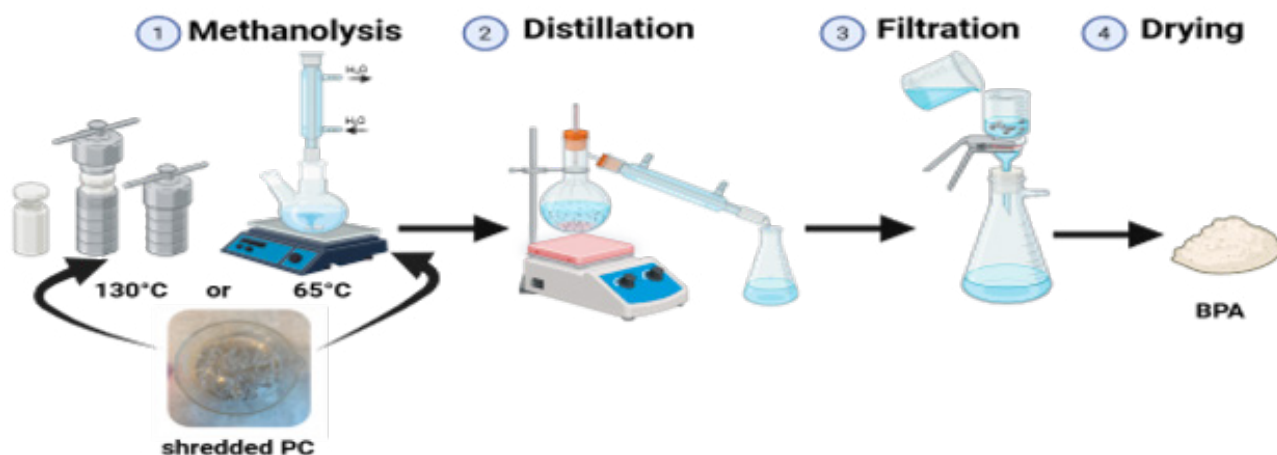
Fig. 18 Scheme of PC methanolysis and monomer recovery
