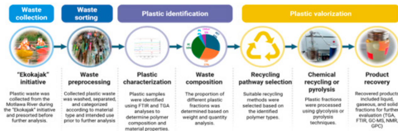
Fig. 3 Workflow for the collection, sorting, polymer identification, recycling-pathway selection, chemical recycling and recovery of products from OBP within the COP project. Created with BioRender.com.
