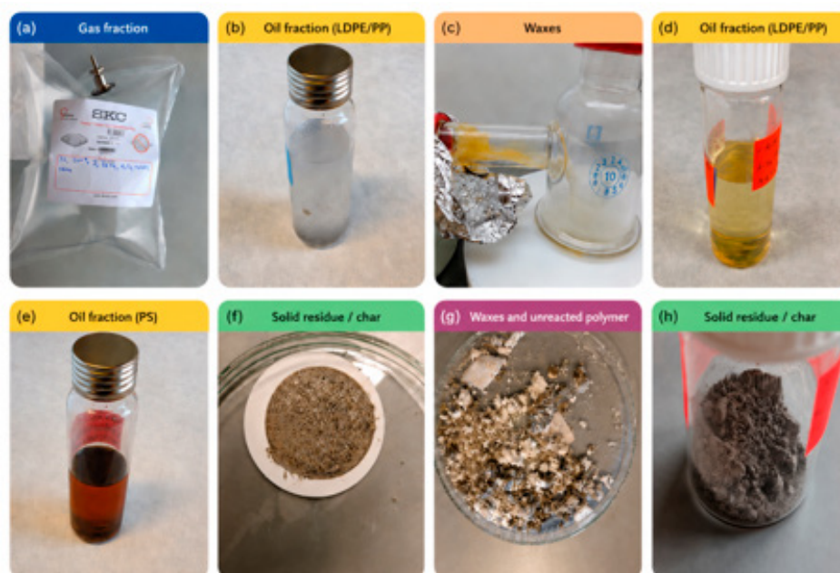
Fig. 23 Representative products recovered after polymer pyrolysis: (a) gas fraction, (b) oil fraction with some waxes/oligomers obtained from LDPE/PP, (d) oil fractions obtained from LDPE/PP, (c) wax deposits collected from the condensation system, (e) oil fraction obtained from PS, (f,h) solid residue/char, and (g) a mixture of waxes and unreacted polymer
