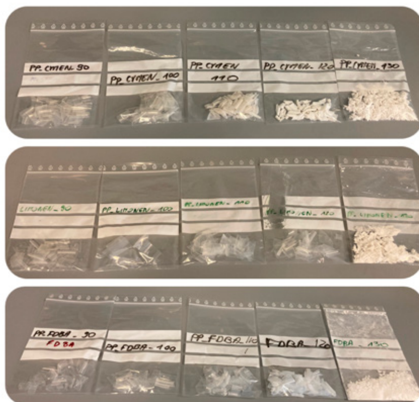
Fig. 8 Effect of solvent type and processing temperature on the visual morphology of PP. Reaction conditions: 5% of polymer, 90-130 °C, time:30 min, solvent to antisolvent volume 1:8.
