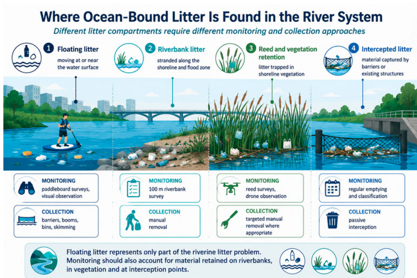
Fig. 2 Monitoring and collection approaches for different compartments of ocean-bound litter in river systems
