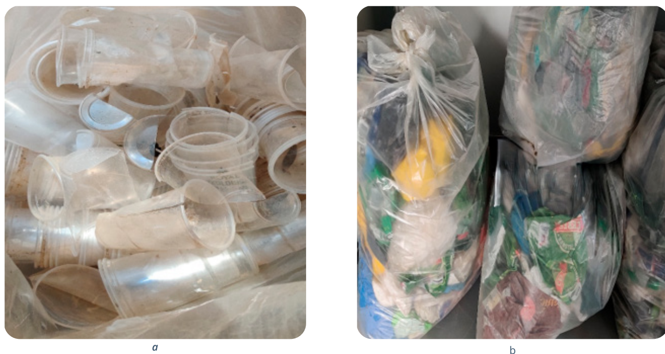
Fig. 1 Selected PP (a) and PE (b) fractions from Aarhus River before pyrolysis. The materials contained visible surface contamination, labels, pigments and other non-polymeric residues.
