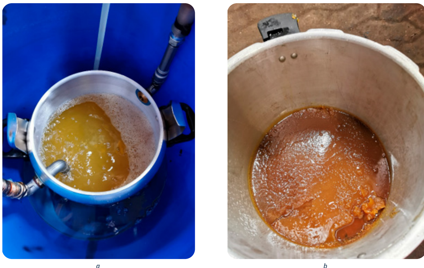
Fig. 3 Examples of condensed oil/wax products collected after pyrolysis. a) Liquid oil/wax fraction during collection and b) heavier wax-like oil product after cooling.
