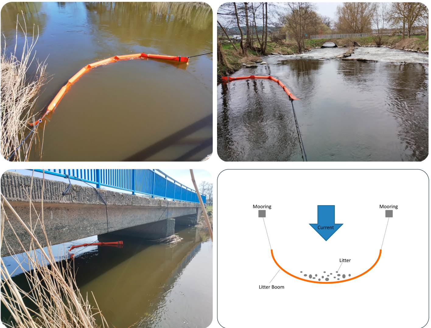
Figure 8: The three locations where the litter boom was tested. (Top left) At the pedestrian bridge in Klein Raden. (Top right) Before the waterfall in Eickhof. (Bottom left) At the Warnow bridge in Baumgarten. Bottom right picture shows a sketch of the litter boom – eagle eye perspective.
